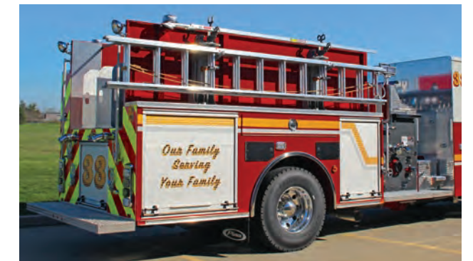
Drop down ladder storage
